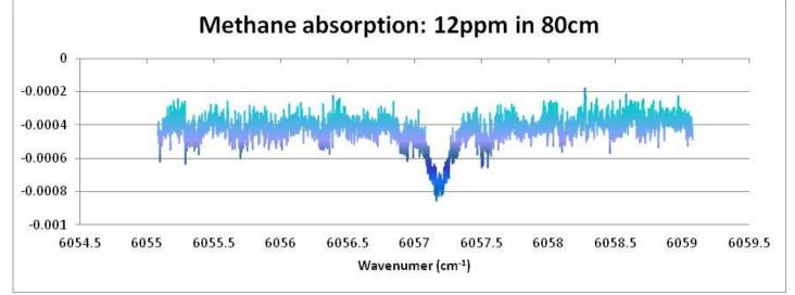
Example of 12ppm concentration of methane in 80cm flowcell. Simulated using HITRAN methane data and actual scanned cell data. Used Aglient 8164A tunable laser to scan line. 0.02% is roughly the noise floor of the laser.
